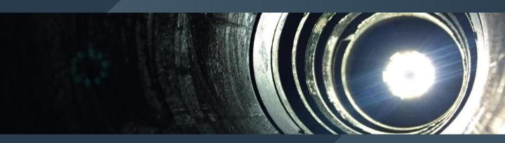
Footage from inside the Camera Overshot showing wireline wrapped around the Fish Top preventing it from entering the fishing grapple.
