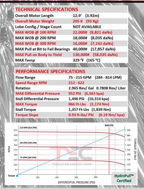
\*\*Performance curves are for reference only. Performance data and dimensions are subject to change without notice. Performance curves based upon Dyno Testing in ambient temperatures, and are dependent on flow rate & power section fit. Actual field performance may vary with field-operational conditions. Operating beyond the parameters given will significantly reduce the longevity of the motor's life and/ or damage.
