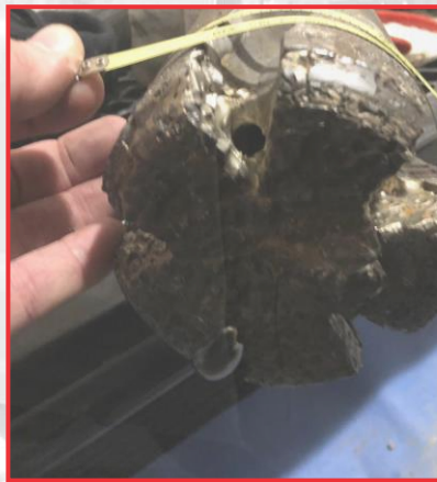
Post Run Mill Pics- only wore down 1.1mm (0.043")!!
