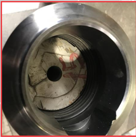
Component from Wireline Setting Tool- P-110 Material
