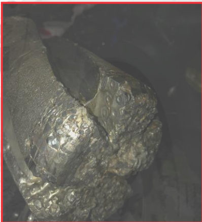
Post Run Mill Pics- only wore down 1.1mm (0.043")!!
