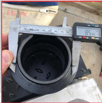
Component from Wireline Setting Tool- P-110 Material
